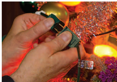
Check to make sure connections are secure and cords are not worn or frayed. Source: Underwriters Laboratories (UL)
